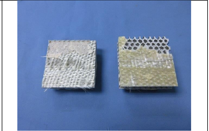
4. Failure mode of sample A
